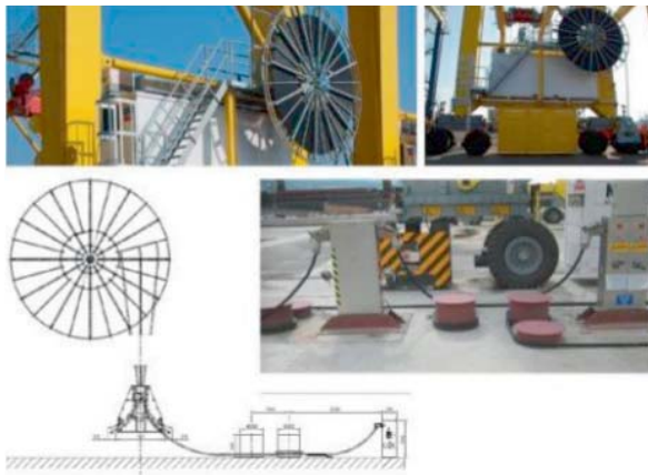
Figure 3 Common type of Cable Reel RTG Electrification System
