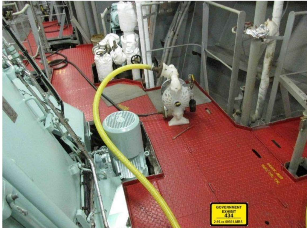
Image showing the so-called “magic pipe” setup. Vessel: Green Sky Credit: DOJ
